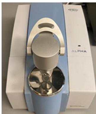
**Bruker: Alpha Fourier Transform Infrared Spectrometer with diamond ATR (Attenuated Total Reflection) (FT-IR ATR)**
