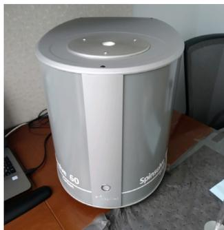
**Magritek: Benchtop 60-Megahertz Multi-Nuclear Magnetic Resonance Spectrometer (NMR):**
