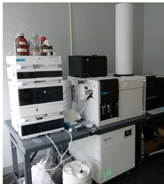
**Agilent: High Performance Liquid Chromatograph with in-line Mass Spectrometer-Time of Flight (HPLC-TOF) (1260 infinity II LC system combined with 6230B Time-of-Flight LC/MS).**
